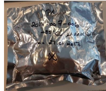
Picture 3: ISO 18936. Each sample is placed in two sealed aluminum bags during accelerated aging.
